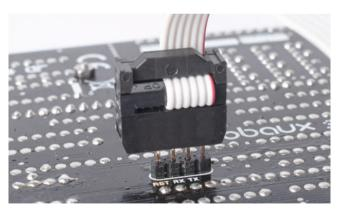
Make sure that the red stripe is pointing upwards, as shown in the picture. The installation is now complete.
