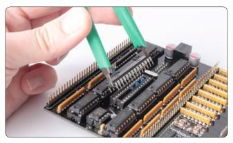
Carefully remove the chip from the main board as shown in the photo.
