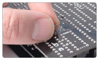
Loosen the small screw located on the lower right side of the back of the module.
