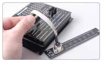
Now put the mainboard back on the module. Press it firmly so that all connections are tight. Connect the adapter to the programmer port.
