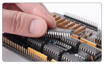
Take the new firmware chip and put it into the empty socket. Make sure that the nose points down as shown in the picture.
